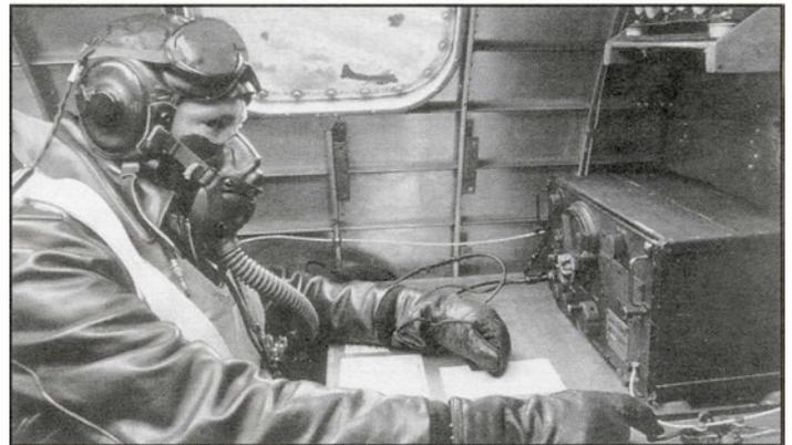
in front of him. The liaison radio receiver and transmitting key were located on the radio operator's table, while the liaison radio transmitter was mounted to the bulkhead directly behind him.
